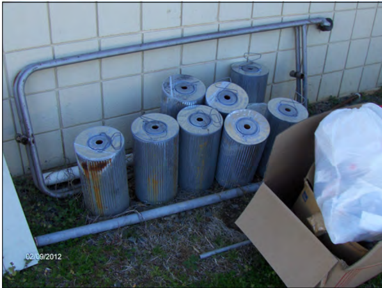
Unacceptable filter storage at a dry cleaning facility.
